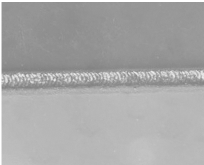
Figure 7: QC picture from the machine vision system of the welding system
