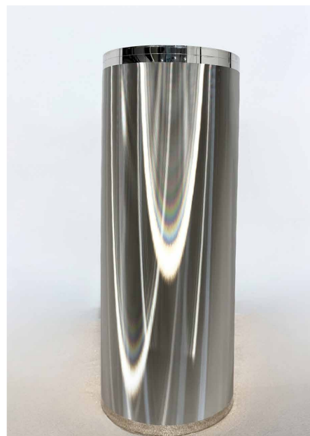
Figure 9: Laser welded sleeve during the optical inspection.
